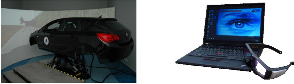
Fig. 3. Research tools intended to be used in the experiments. Left: AS1200-6 simulator. Right: SMI Eyetracking Glasses 1.8 mobile eyetracker.
