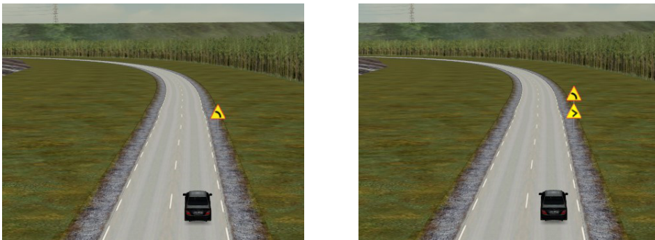
Fig. 4. Example of an experimental road situation. Left: road curve with classical signing. Right: road curve with an experimental sign supplementing the classical sign.
