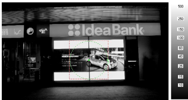
Fig. 4. The search for value L_{max} [ cd / m^2 ] in one field of measurement (126000 pix).
