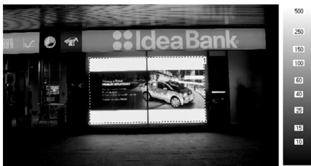
Fig. 6. The search for value L_{max} [ cd/m^2 ] using the meter matrix (318750 points - reference value).
