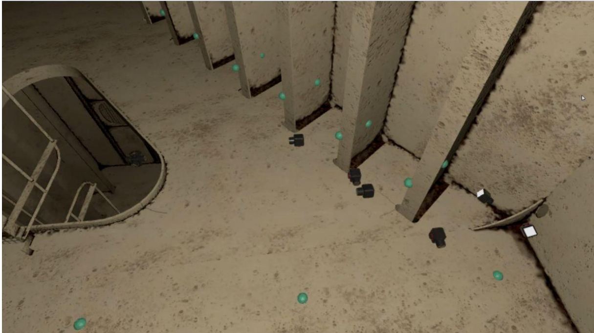
Fig.6: Indication of thickness measurement points and camera positions for close-up imagery viewed in VR
