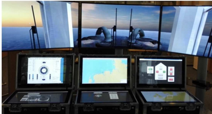
Fig.5: Mobile Bridge in the Virtual Testbed
