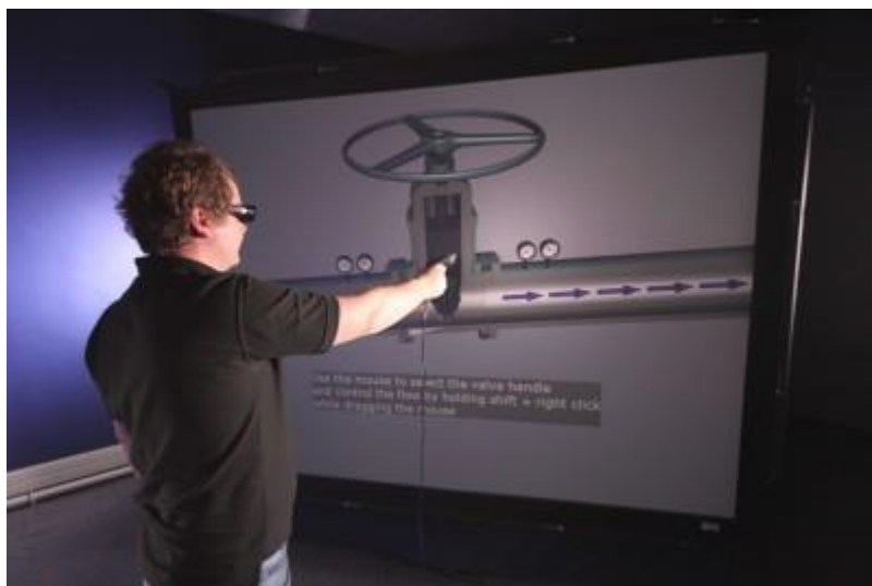
Fig.8: Customizations in VR software can be used to add animations for training, e.g. valves turning
