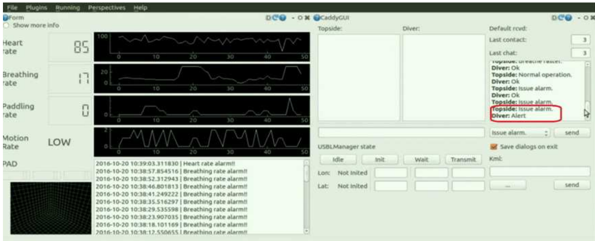
Fig.14: Remote station console used to monitor diver physiological state and to communicate via chat messaging service
