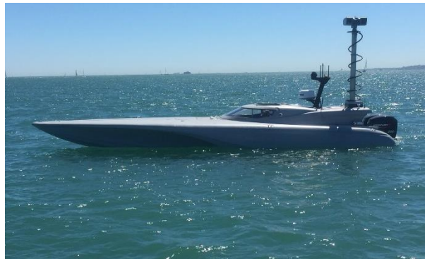
Fig.1: The MAST platform is a 34ft Bladerunner racing hull retro-fitted with ASV control system and extensive additional testbed hardware and software
