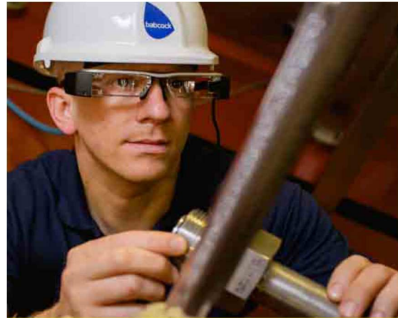
Fig.22: Smart glasses will allow hands-free operation in assembly and operation, Patterson and Webb (2016)
