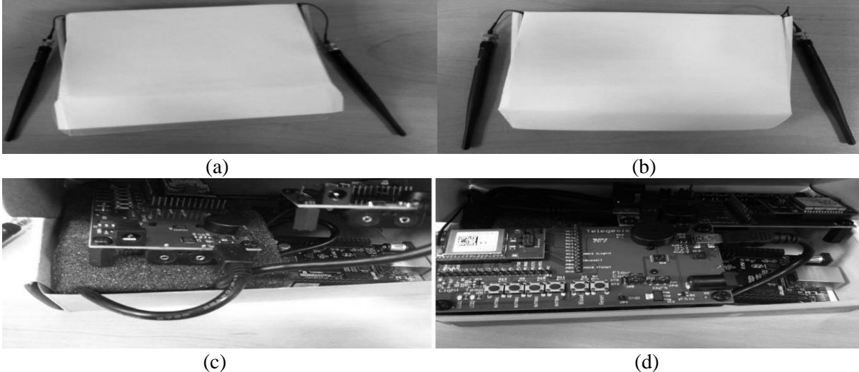
Fig.5: Four SmartDAQs with virtual sensors: (a) and (b) housing and antennas, (c) and (d) wireless transmitter development boards and embedded Linux boards, battery powered.
