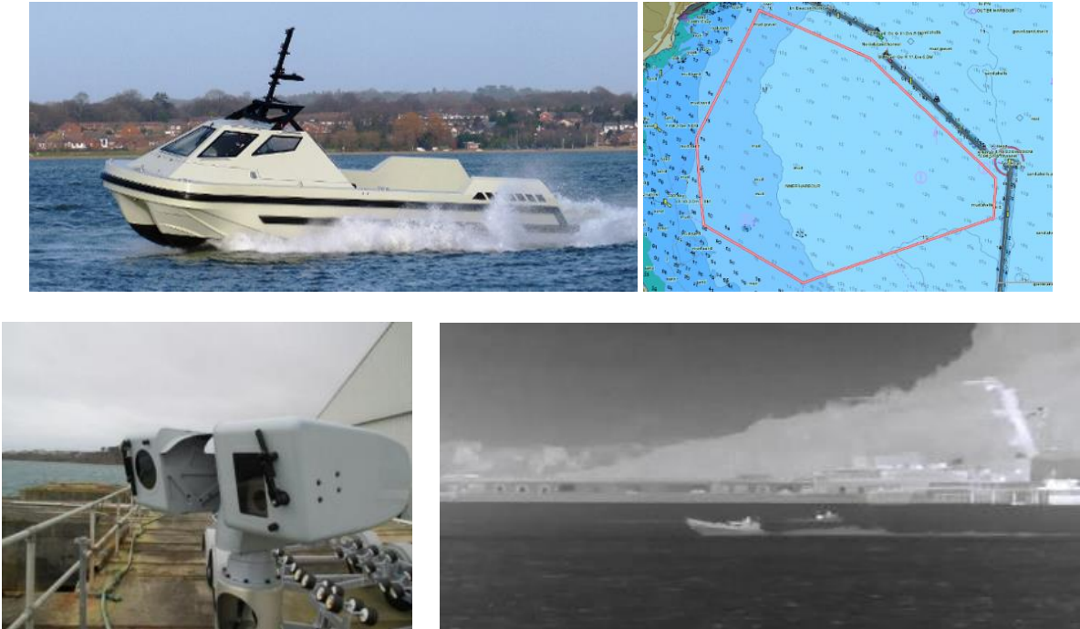
Fig.7: ARCIMS USV (top-left); sea-trial controlled environment (Bingleaves/UK) (top-right); Electro Optical camera (bottom-left); EO image (bottom-right).
