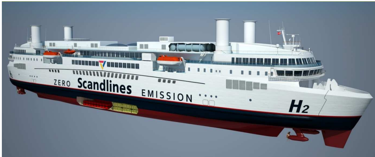
Fig.9: Zero-emission ferry design with fuel cells and batteries, supplemented by Flettner rotors harnessing wind energy, Rohde et al. (2013)
