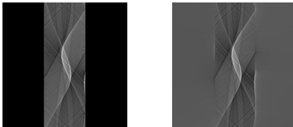
Fig. 6. The sinogram with empty areas and the sinogram where those areas filled with edge values.
