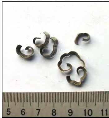
Figure 199: Type of chip obtained in the machining tests for the 18CrMo4 with standard and with ultra fine grain size.
