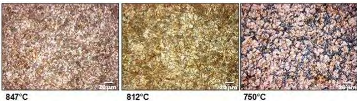
Figure 116: Microstructure of water cooled specimens of steel 18MnB2 versus finish rolling temperature.
