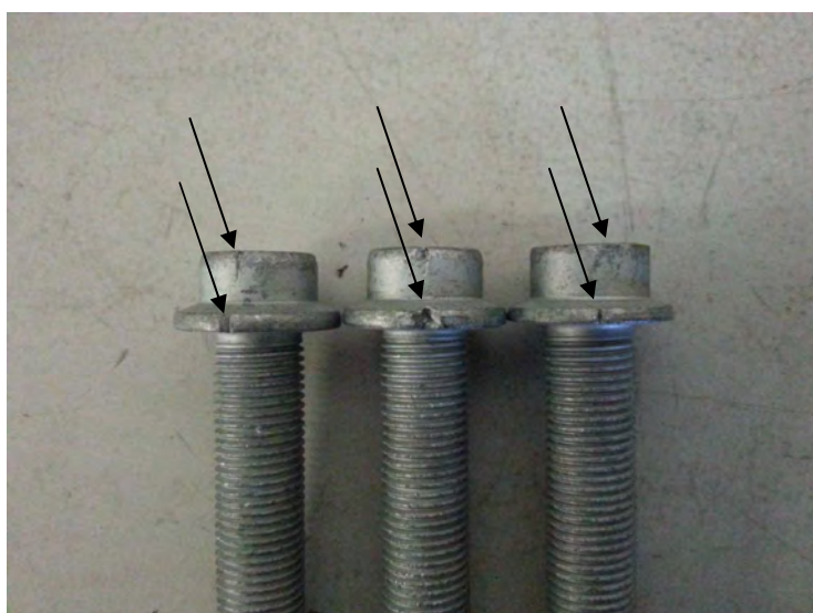
Figure 201: M14 screws rejected for defects originated by pre-existing surface defects.
