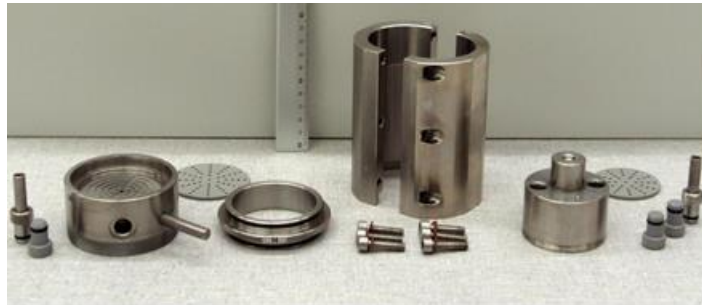
Figure 8-3: Disassembled sample cell with the two removable sidewalls for uniaxial testing.
