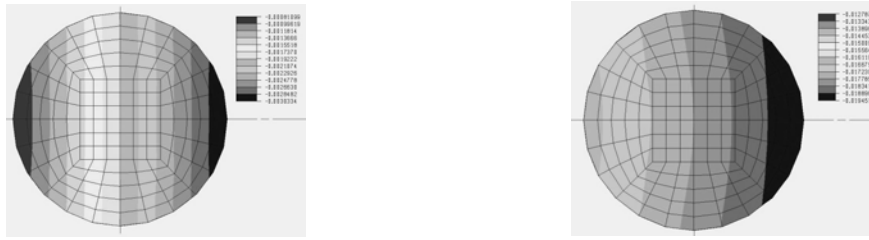
(a) Elastic stage (0.18% compression) (b) Elastic stage (1.5% compression) Figure 16: Comparison of Distribution of strain in elastic stage and plastic stage
