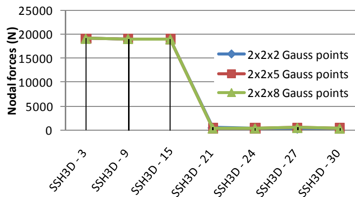
Figure 10: Nodal forces for the isochoric deformation mode of Figure 6 (d) (warp mode) versus the number of EAS modes in the SSH3D element for three different integration schemes.
