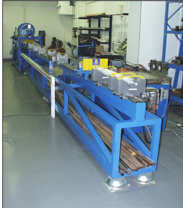
Figure 2: SHTB setup at Ghent University. Its total length is 11m.
