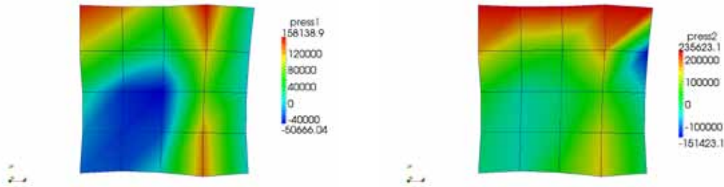
Figure 3: Macroscopic distribution of two perfusion pressures p_1 and p_2 in the deformed domain \Omega (evaluated at the final time of the simulation).
