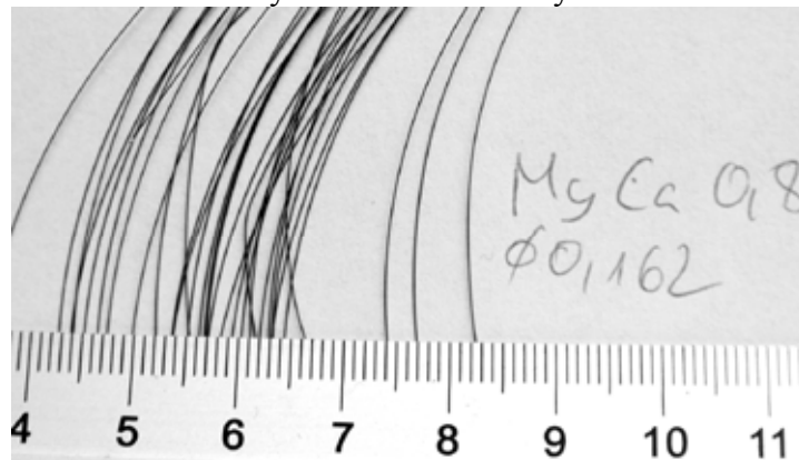
Figure 6: Wires from MgCa08 after drawing, d=0.16 mm
