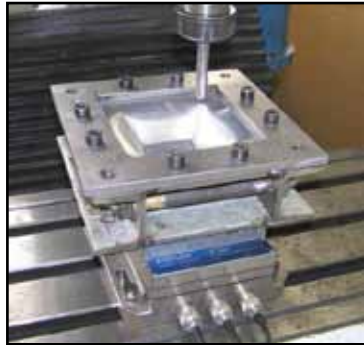
Figure 2: The experimental equipment for SPIF experiments (three-axis milling machine tool - SPIF tooling system) [17]
