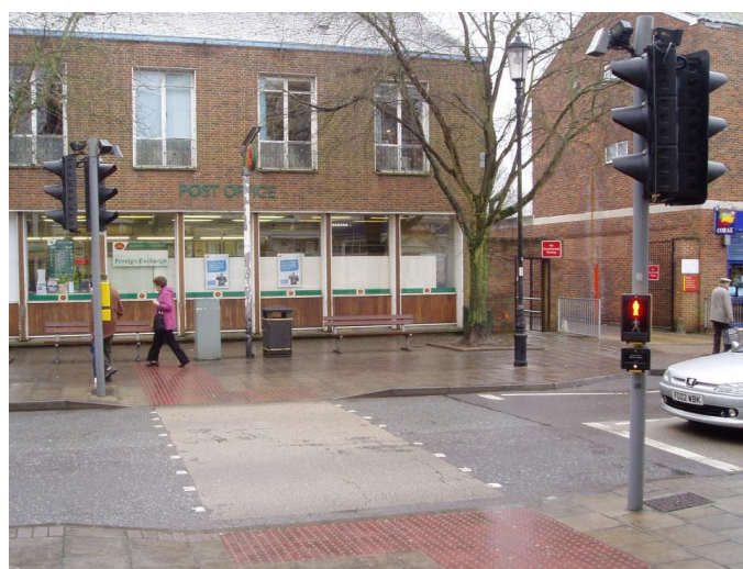
Figure 2.1: Example of a mid-block Puffin crossing
