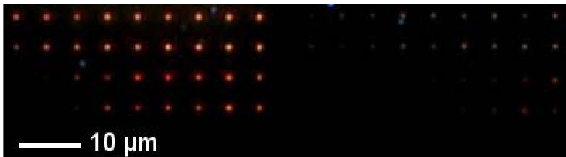
Figure 6.2: Real colour CCD image of the longitudinal scattering response of two-arm (left, nominal gap size 20 nm) and single-arm (right) gold nanoantennas with arm lengths of 25 nm through 65 nm (lower two lines) and 70 nm through 110 nm (upper two lines), with each arm varied in 5 nm steps.
