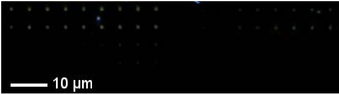
Figure 6.3: Real colour CCD image of the transverse scattering response of two-arm (left, nominal gap size 20 nm) and single-arm (right) gold nanoantennas with arm lengths of 25 nm through 65 nm (lower two lines) and 70 nm through 110 nm (upper two lines), with each arm varied in 5 nm steps.
