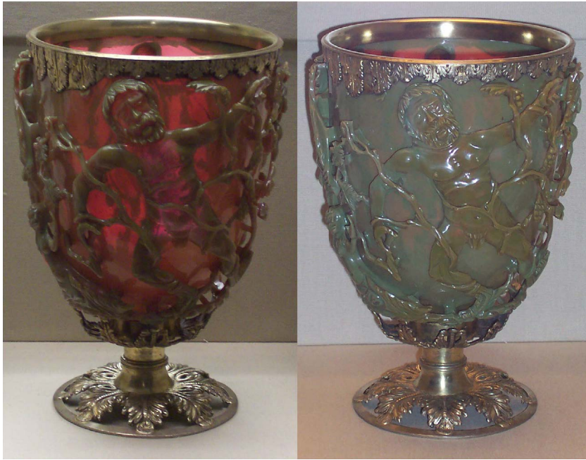
Figure 2.9: The Lycurgus Cup when photographed without (left) and with (right) the use of a flash. In the first image, the transmission contribution is dominant, in the second, the scattering contribution. (Photographs from a personal visit to the British Museum)
