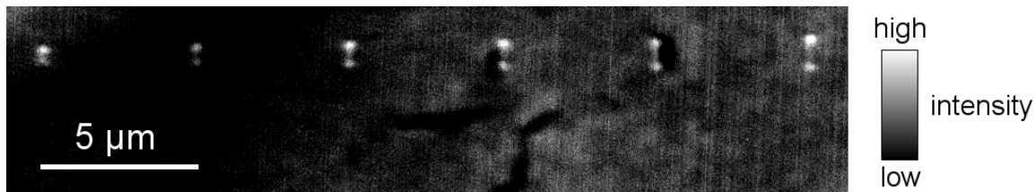
Figure 9.7: Raster scan image as recorded by the single-photon detector for a quantum dot (QD) excitation with laser light polarized along the long rod axis for rods of total length 500 nm (left) through 1 \mu\text{m} (right). The emission is clearly enhanced at the rod ends as already seen in the TPL experiment. No explicit rod length dependency is recorded. Only a qualitative emission intensity scale is given, as the exact emission intensity depends significantly on the quantum dot layer concentration at specific points, such that no quantitative value on the emission enhancement can be calculated from the recorded images. The fact that the distribution and emission of the QDs is not the same all over the sample is seen by additional shapes imprinted in the luminescence response.
