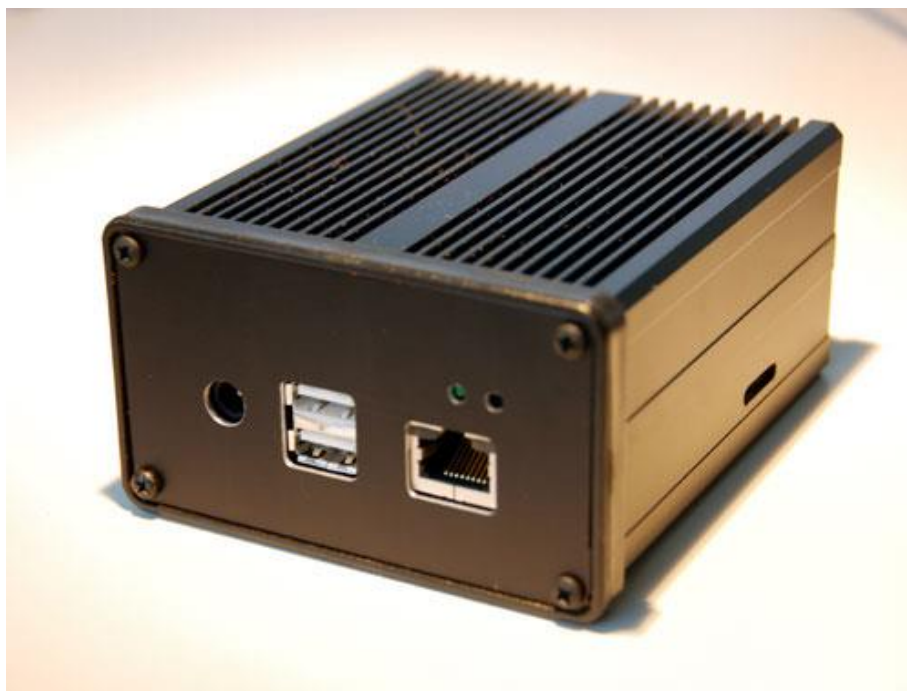
Bild 16: Wireless Data Concentrator (WDC)
