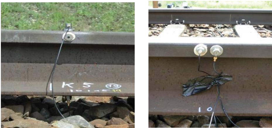
Fig. 26: Two accelerometers, Ch1 and Ch2, were used simultaneously during the whole measurement campaign to evaluate the effects of mounting and position.
