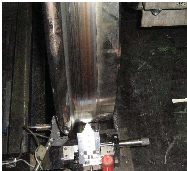
Fig. 54: Sensor of the wheel roughness measuring device on the running surface of a test wheel.
