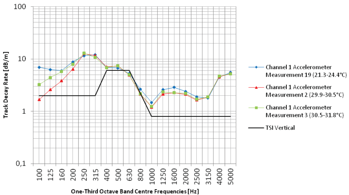
Fig. 29: The vertical decay rate measured at starting point K2. Comparison of two repeated measurements (natural variation) with a third measurement performed at a different day and with 5-10°C temperature change.
