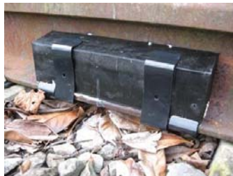
Fig. 84: Silent Track ® damper manufactured by Tata installed on the test track
