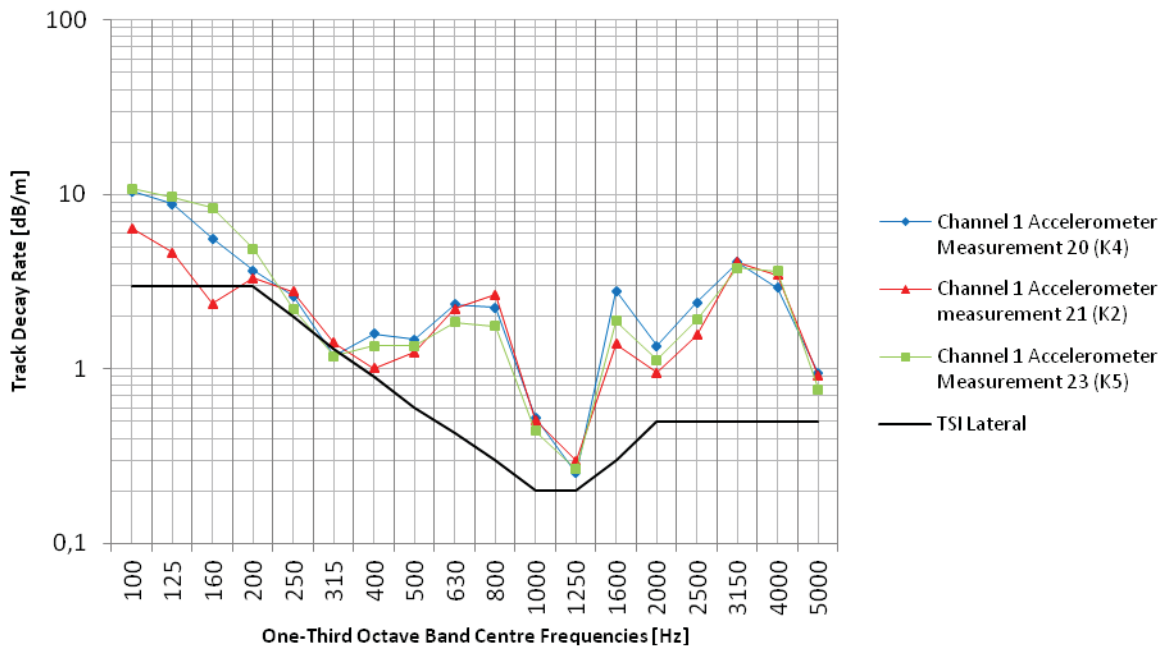
Fig. 35: Lateral TDR measured at three different positions along the right hand rail.
