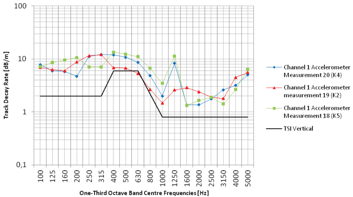
Fig. 34 : Vertical TDR measured at three different positions along the right hand rail.
