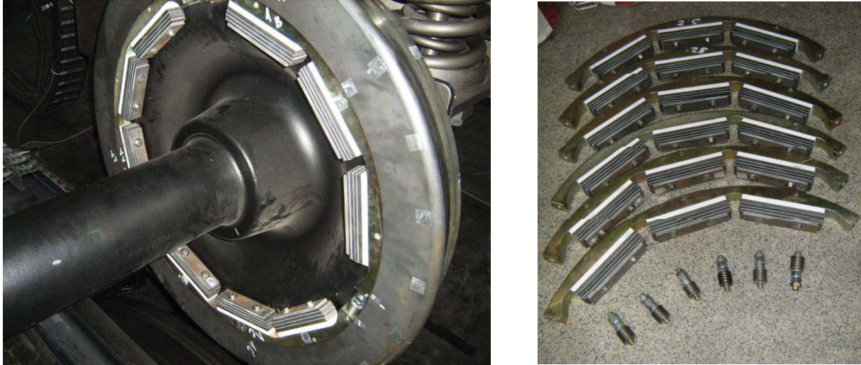
Fig. 52: Left: Wheel BA 308 equipped with wheel damper of type Vicon-Rasa (Schrey und Veit); Right: Individual damper assemblies. Each wheel needs three assemblies to cover the full circumference.
