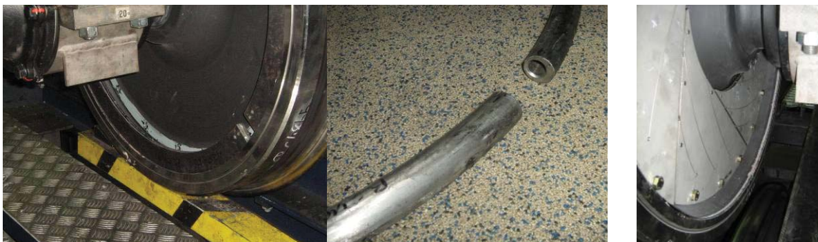
Fig. 53: Left: Wheel LK900 with the DAAVAC wheel damper (Pinta-Enac); center: ring damper (Valdunes); right: plate damper (GHH Radsatz).
