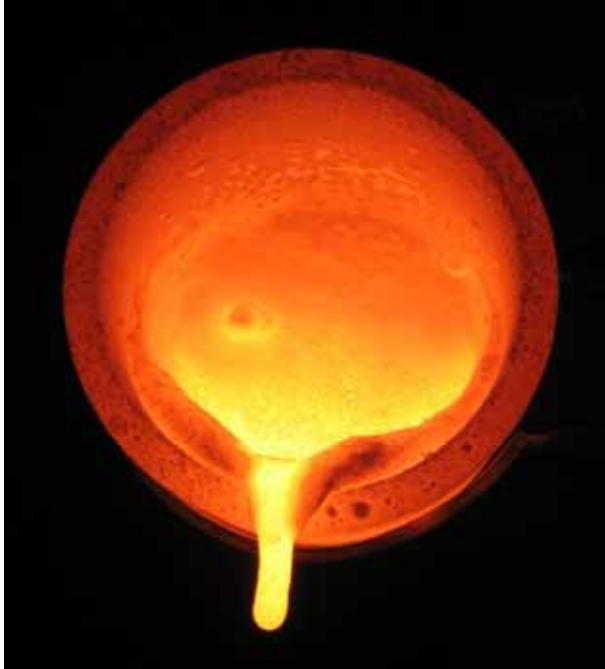
11.2c: \text{Al}_2\text{O}_3 = 8,8 \text{ M.-%} \eta_{1500^\circ\text{C}} = 1081 \text{ mPa s}
