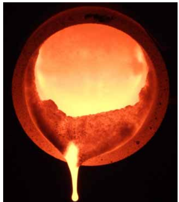
11.3a: C/S = 1,42 \eta_{1500^{\circ}\text{C}} = 737 \text{ mPa s}
