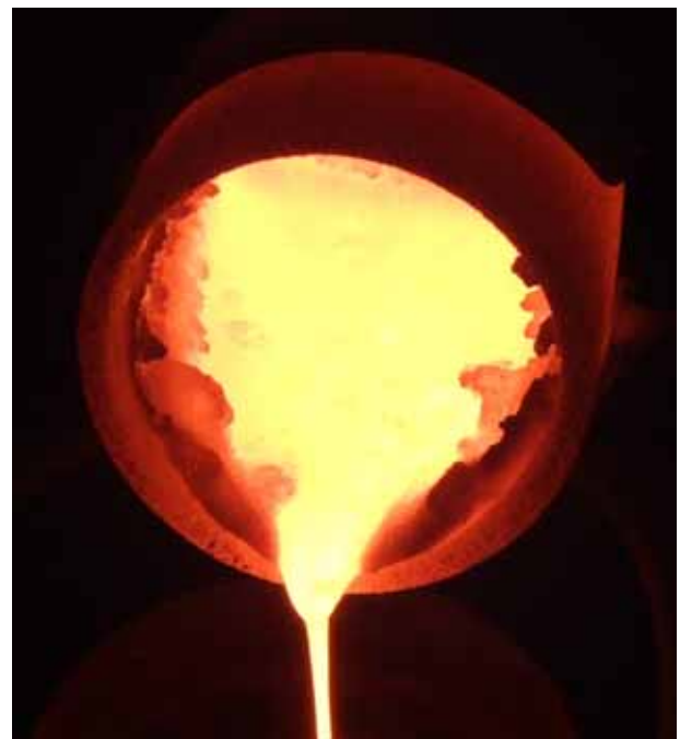
11.2b: \text{Al}_2\text{O}_3 = 21,6 \text{ M.-%} \eta_{1500^\circ\text{C}} = 919 \text{ mPa s}
