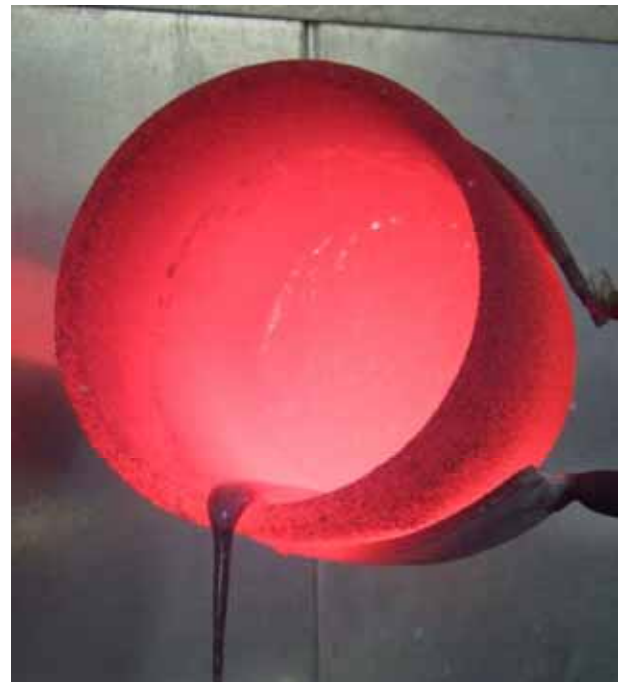
11.3b: C/S = 1,00 \eta_{1500^{\circ}\text{C}} = 923 \text{ mPa s}
