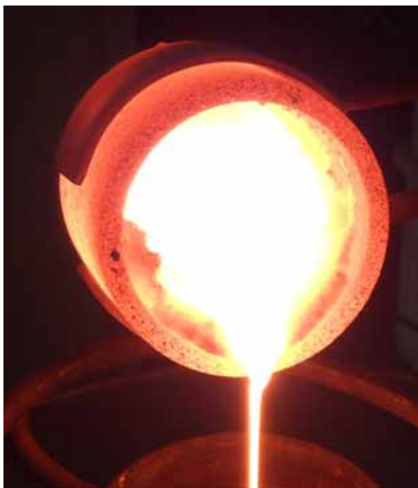
11.0: C/S = 1,22 \eta_{1500^{\circ}\text{C}} = 655 \text{ mPa s}
