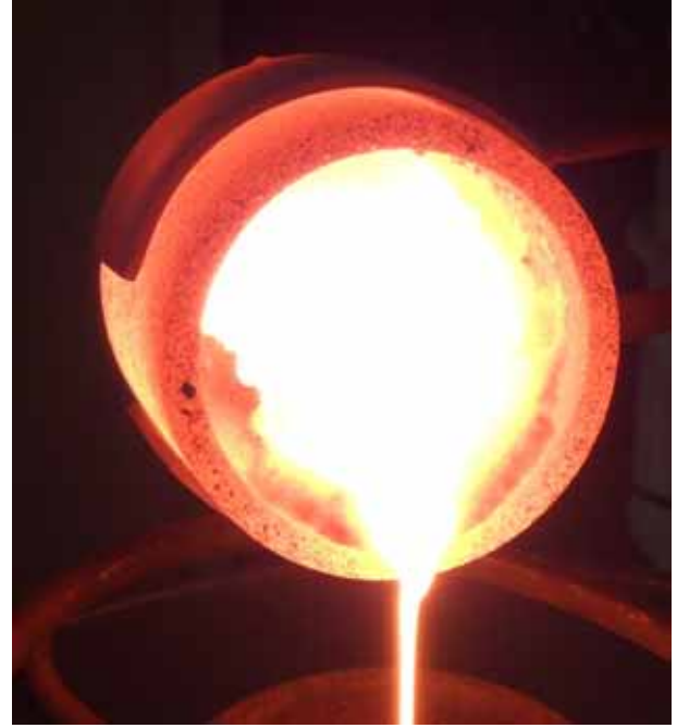
11.0: \text{Al}_2\text{O}_3 = 11,4 \text{ M.-%} \eta_{1500^\circ\text{C}} = 655 \text{ mPa s}
