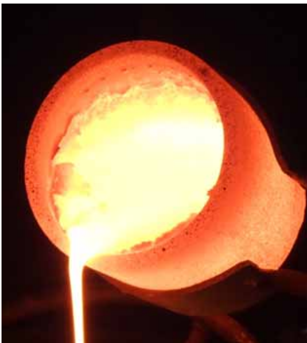
11.2a: \text{Al}_2\text{O}_3 = 18,2 \text{ M.-%} \eta_{1500^\circ\text{C}} = 634 \text{ mPa s}
