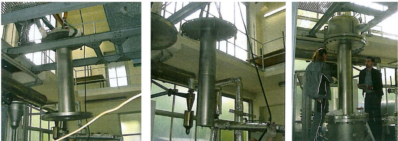
*Figure 5.3:: Middle part of the ESP, Collecting electrode, Installation of the filter head*
