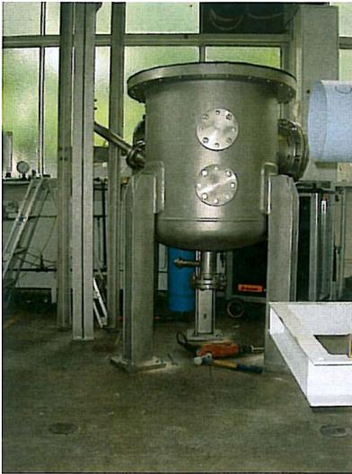
*Figure 5.2: The bottom of the tar-ESP was set into position at TU Berlin*
