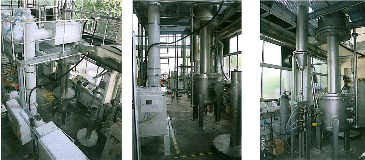
Figure 5.4: General view of the plant (ESP and Quench), incl. HV-unit, switch cabinet
