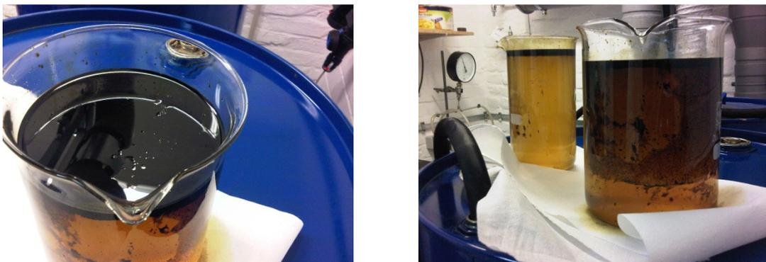
Figure 5.9: Tar-RME-Water mixture from ESP outlet
