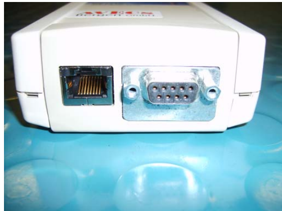
RJ45 Network connection
