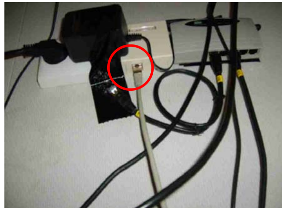
Bypass Cable connection in case of switch error
