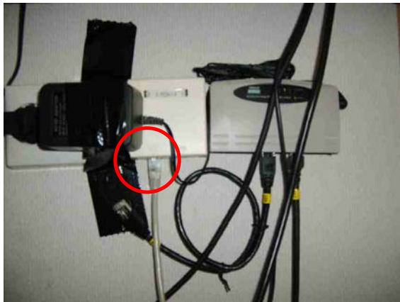
Bypass Cable connection in case of switch error
