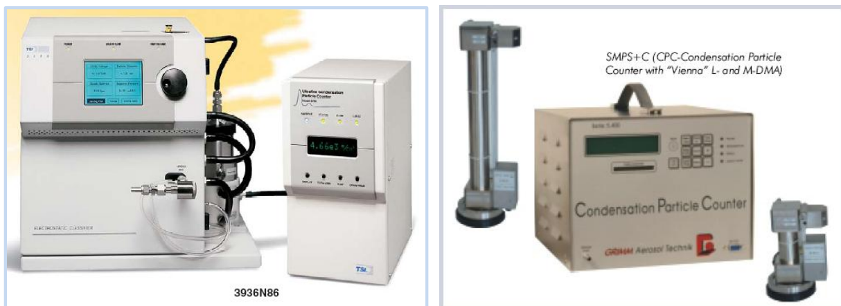
Figure 17. Examples of typical SMPS systems manufactured by TSI Inc (left) and Grimm Aerosoltechnik GmbH (right).
