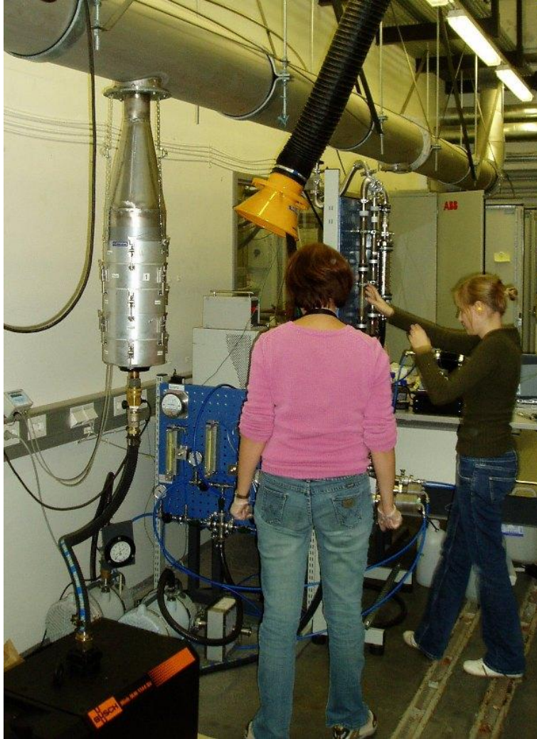
Figure 18. Size-segregated particulate collection using a high-volume (850 litres/min) cascade impactor (HVCI) connected to a dilution tunnel, in which there was a 200-fold dilution of the flue gas from a log wood batch burning device.
