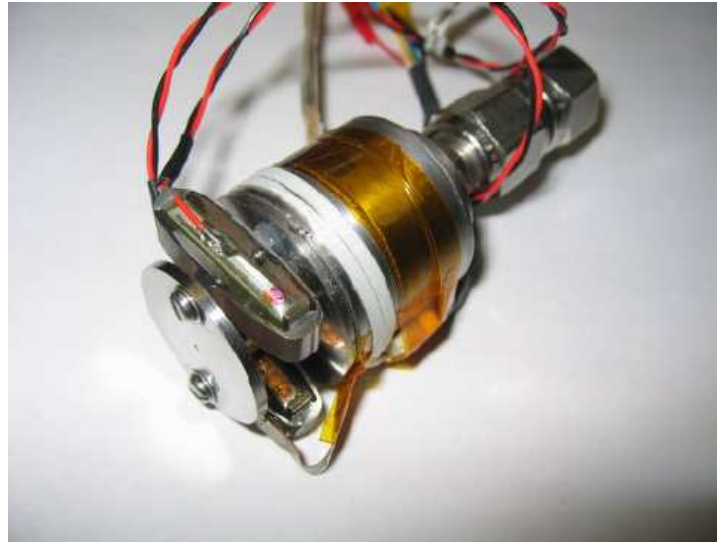
Figure 13: Micro Thruster Assembly (image by Bradford Engineering)
