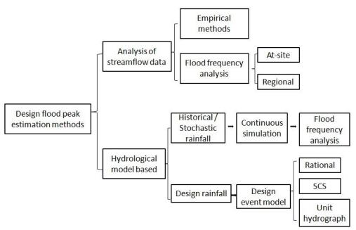
Figure 1.2: Approaches to design flood peak estimation
