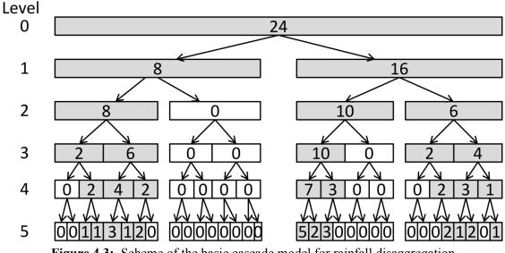
Figure 4.3: Scheme of the basic cascade model for rainfall disaggregation (modified from Müller and Haberlandt 2015)
