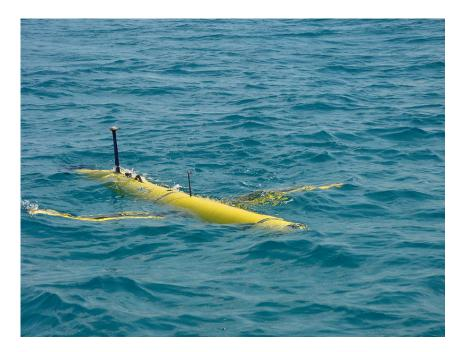
Figure 2.5: Bluefin-12 UUV with a Buried Object Scanning Sonar (BOSS) integrated in two wings
