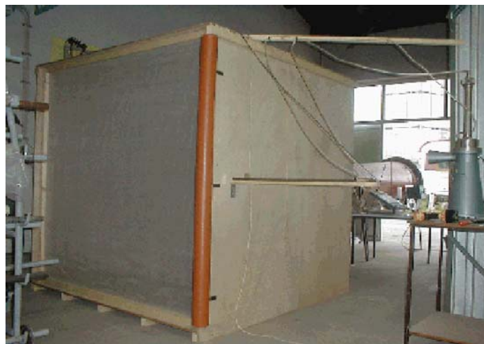
Figure 3.2.2: A photograph of the wind tunnel used to measure the pressure drop across the insect-proof nets. An insect-proof net can be seen placed on the end of the wooden box ready for measurement. The fan is located at the end of the cylindrical duct.
