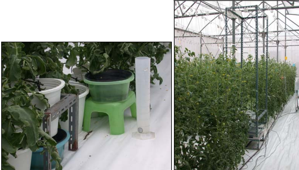
Figure 3.5.1: Measurement of plant water consumption: the manual measurements of dripper solution and leachate, collected in separate buckets (left) and the lysimeter with an electronic balance used to measure evapotranspiration (right) inside the greenhouses in Central Thailand.
