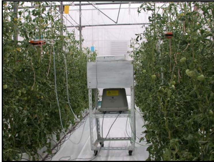
Figure 3.7.3: Experimental setup of the online measurement of plant response in the greenhouses in Central Thailand. The leaf cuvettes (with one or several leaves inside) were placed in a horizontal position and connected to the mixing chamber using small pipes.
