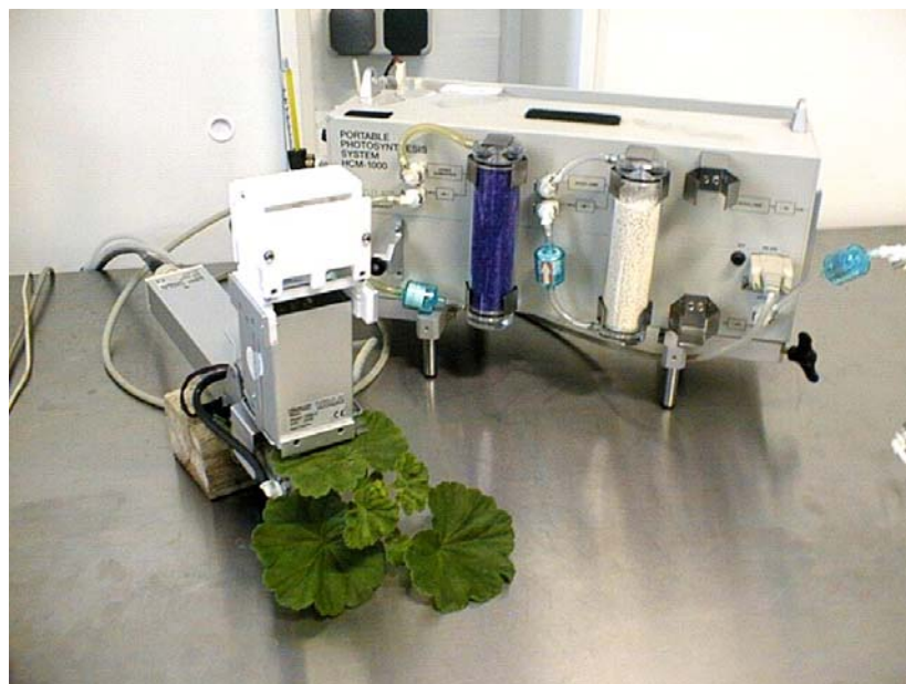
Fig. 2A. Picture showing the device for measurement of photosynthetic rate (Portable Photosynthesis System, HCM-1000)
