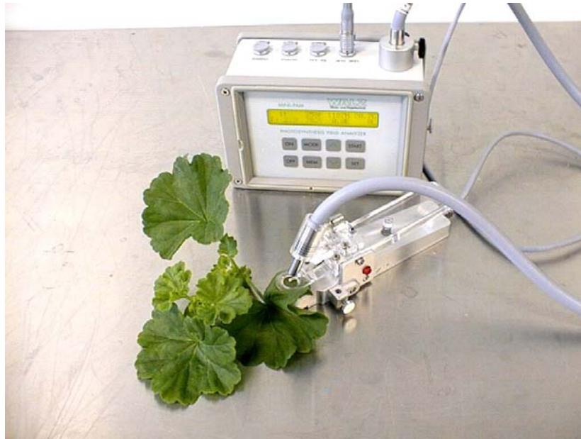
Fig. 1A. Picture showing the device for measurement of chlorophyll fluorescence (Photosynthetic yield analyzer MINI-PAM).
