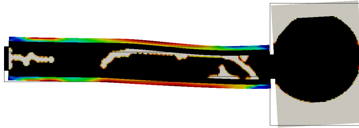
Figure 5.19.: Applying the modified Heaviside filter (A.4) to the stress constrained model with reinforcement. The converged result for the Heaviside parameter \beta = 256 is shown. J_{\text{power}} is improved by 64% (the highest obtained value), \sigma_v is 2.5% below the stress of the solid resonance case.
