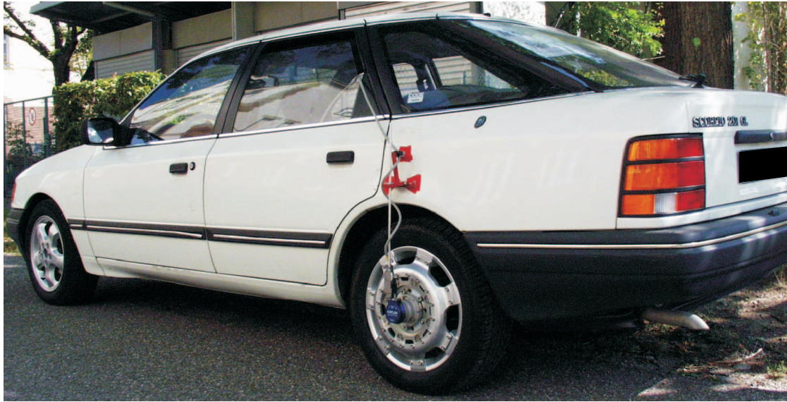
Figure 6.2: Test vehicle with wheel torque sensor
