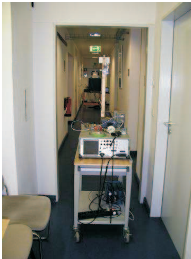
Figure E.1: Corridor type I: 1.3 \times 13.07 \times 2.57 m.
