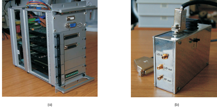
Figure 4.1: (a) Digital array transceiver: eight IF inputs at 200 MHz, 10 bit resolution with the sampling frequency of 16 MHz, data transfer to PC over EPP interface, (b) Tx modulator with an external LO input and an IF output.
